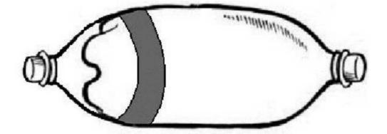
4. Add some kind of ballast into the space between the cut neck and the intact bottle. Beans or rice work the best.
